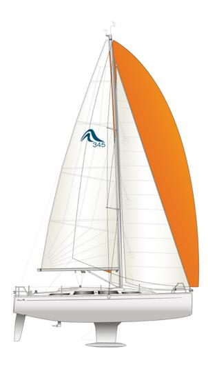
10.40 m | 34′1″ Hull length 9.99 m | 32′8″ LWL 9.55 m | 31′3″ Beam 3.50 m | 11′5″
