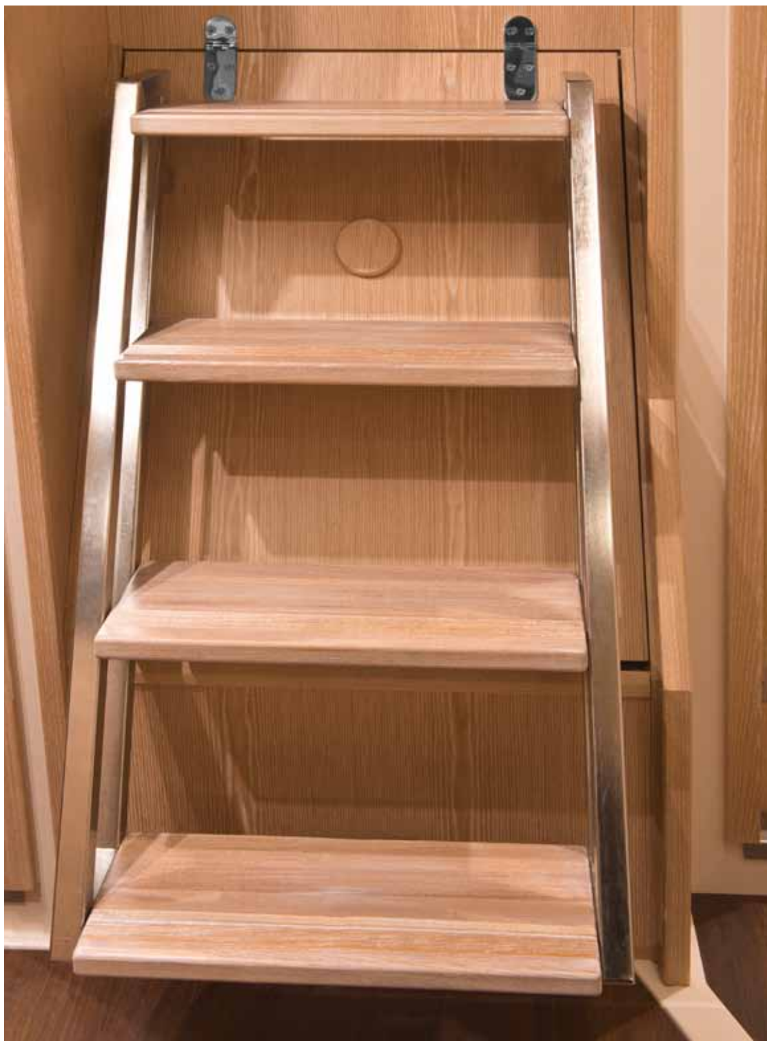
2 Comfortable and well designed: New companionway with a 7° flatter stair angle.
