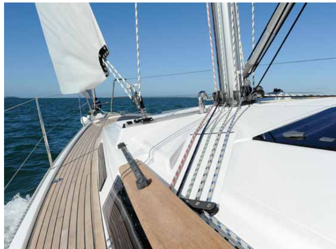
3 One step coach roof design leads aft with all ropes covered.
